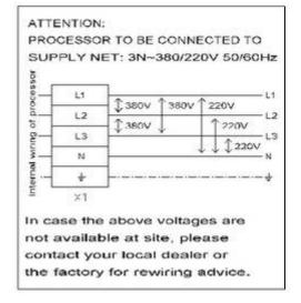
Alternative, the processor can be installed using 3x220V 50/60 Hz supply net - this has to be indicated accordingly when ordering.
