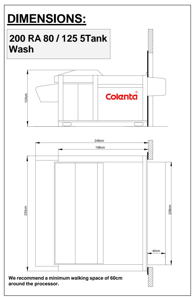
Specifications for wall-opening when the processor has to be installed that way.
