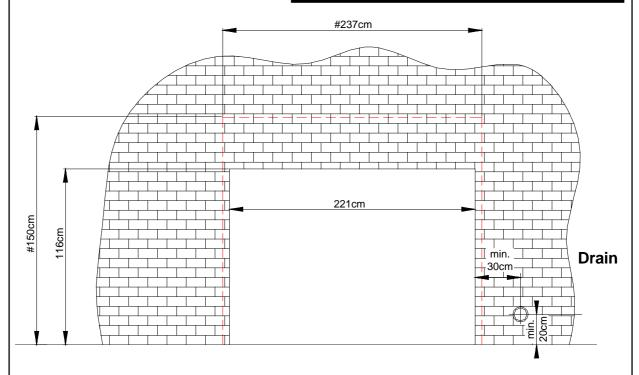
In case the thickness of the wall is more than 2cm, the cut-out of the wall has to made according the measurements marked with # - in that case a panel has to be installed as well, this to keep the cover lid of the processor in position - as shown below:
