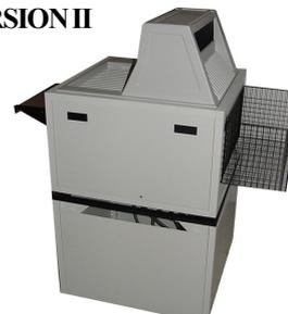
All **Colenta Mediphot** X-Ray processors provide a full automatic „dry to dry“ film processing technology. A microprocessor system ensures precise temperature control of all processing chemistries with automatic Developer / Fixer tank cooling to prevent overheating. Replenishment is preheated by injection into the inline chemical heating system, which is controlled to pre-set programmed temperatures within +/- 0,2 °C.
